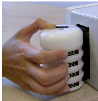
Figure 1. Braille stimulators are placed inside five stacked disks. The disks of the cylinder could be rotated individually to adjust optimal placement of the Braille stimulators on the fingers of the subject, when he grasped the cylinder.
