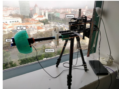
Fig. 3: Previously built biomimetic 3D eye model. It is composed of a supportive green eye mounted on a ball joint sustained on a tripod. The eye is connected to six elastics (representing the six extraocular muscles) and controlled by three motors that pull the endpoints of those elastics (commanding, thus, only each pair of antagonist muscles) [14].
