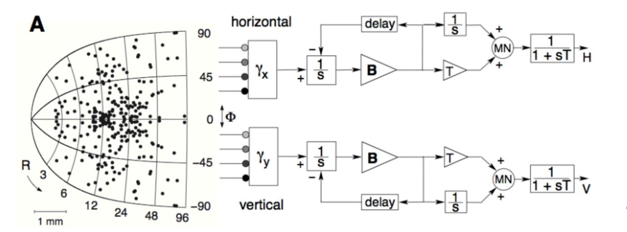
Fig. 5: Our computational optimal control model of how monkey SC (motor map on left) encodes the kinematics and trajectories of eye saccades. The model is driven by measured spike trains from  $\pm 150$  SC cells [19,20].
