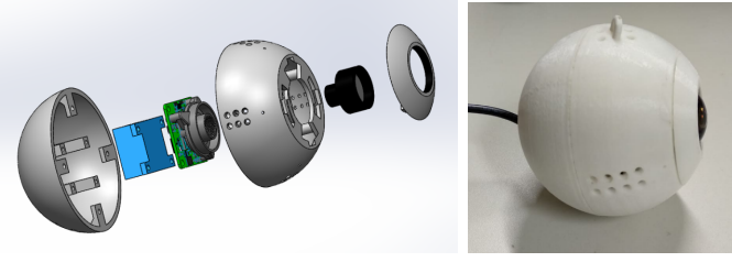
Fig. 3. Left: Exploded view of the CAD model of the eyeball with the IMU, camera and lens. Right: Side view of the final eyeball showing the holes for potential cable insertion point.
