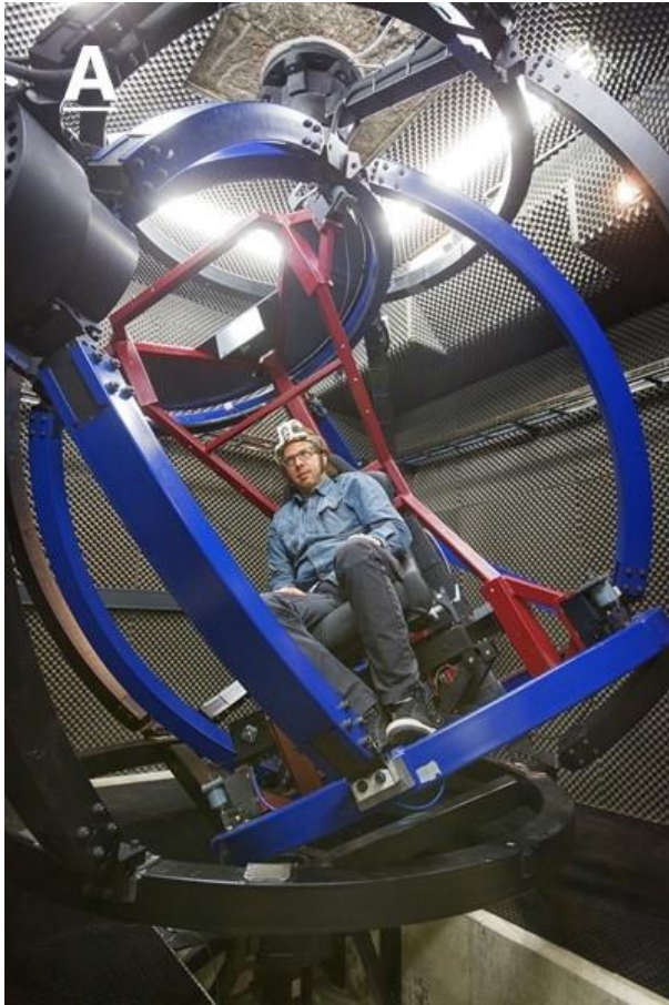
Figure 4 – A: This image shows the structure of vestibular chair. The black beam structure can be rotated about the vertical axis and the blue beams can be rotated about the horizontal axis. ( www.ru.nl ) B: This image shows the hemisphere of the 63 speakers and LED's with the middle one being the fixation LED. ( www.mbfys.ru.nl )
