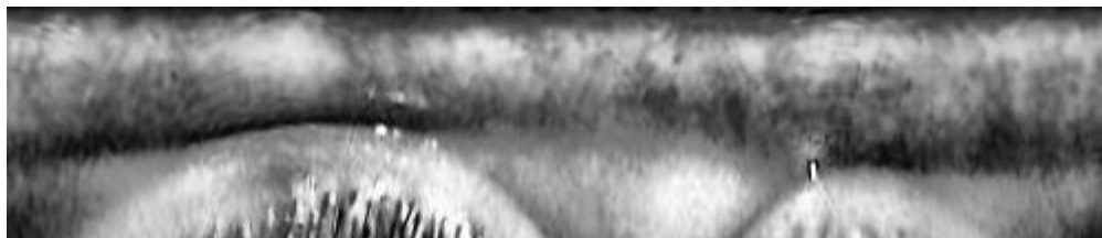
Figure 7: A polar plot made by extracting the enlarged ellipse surrounding the pupil and applying an affine transformation that transforms it into a circle. The largest part of the pupil on top is extracted and the number of pixels on the vertical axis is set to 500 (using linear interpolation). The entire horizontal axis corresponds to 2\pi
