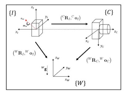
$R_k$  – Orientation  $v_k$  – Linear velocity  $o_k$  – Position  $b_k^{g,a}$  – Biases (gyroscope and accelerometer)  $p_1 \dots p_p$  - Landmark positions
