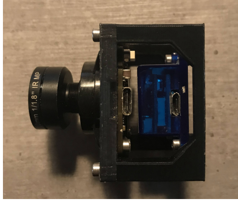
Figure B.6: Visual-inertial sensor configuration used.
