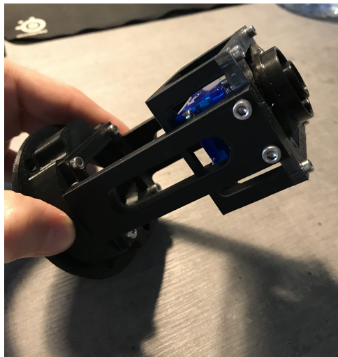
Figure 1.3: Eye system with camera and inertial sensor. This setup is just a replica of the actual eye prototype and was used for benchmarking purposes as will be shown later in section 4.3.1.
