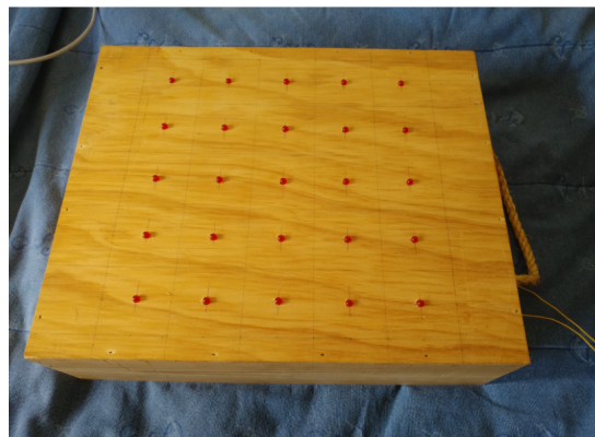
Figure A.4: (a) Schematic used for the connection of the LEDs, and (b) LED pattern in a rigid surface for calibration
