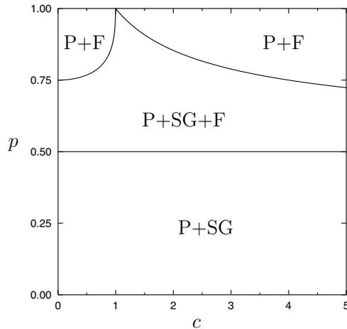
**Figure 5.** The possible phases of the ‘small world’ spin glass for the different allowed combinations of the dimensionless control parameters  $c \geq 0$  (the average Poissonian connectivity) and  $p \in [0, 1]$  (the probability of  $J_{ij} = +J$  in the Poissonian bonds).
