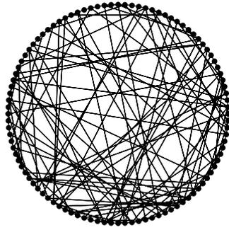
**Figure 1.** Example of a ‘small world’ lattice connecting  $N$  spins (indicated by  $\bullet$ ) in the sense of our present models. Nearest neighbour interactions along a one-dimensional ring are combined with sparse long-range interactions in the form of a random Poissonian graph, with small average connectivity  $c$ . Here  $N = 100$  and  $c = 2$ .
