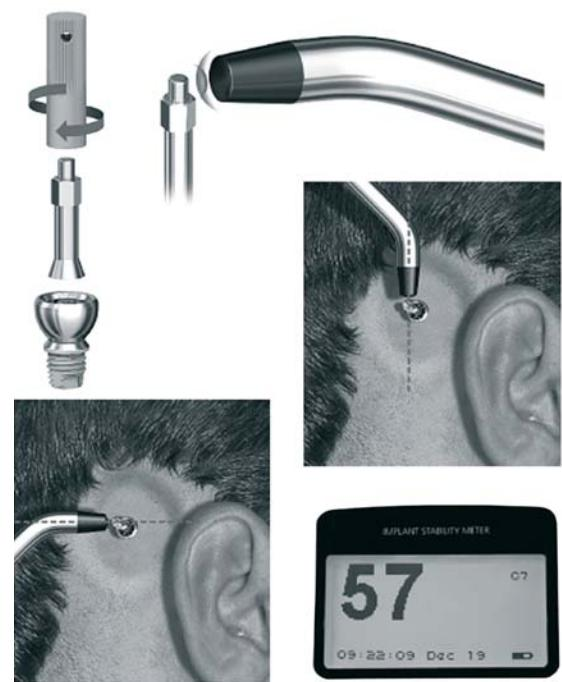
Resonance frequency analysis (RFA). First, the SmartPeg is screwed on the abutment. Second, the handheld electronic analyses device excites the SmartPeg through electromagnetic pulses and analyses the implant stability quotient (ISQ). Figures courtesy of Osstell AB and Cochlear Bone Anchored Solutions AB.)
