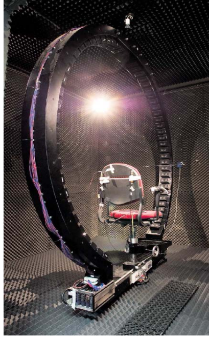
Figure 2.1. Experimental setup. Anechoic, sound-attenuated room, which contains a hoop with 58 speakers attached. Three orthogonal magnetic fields in the corners of the room induce alternating voltages in the dual search coil mounted on the subject's head.
