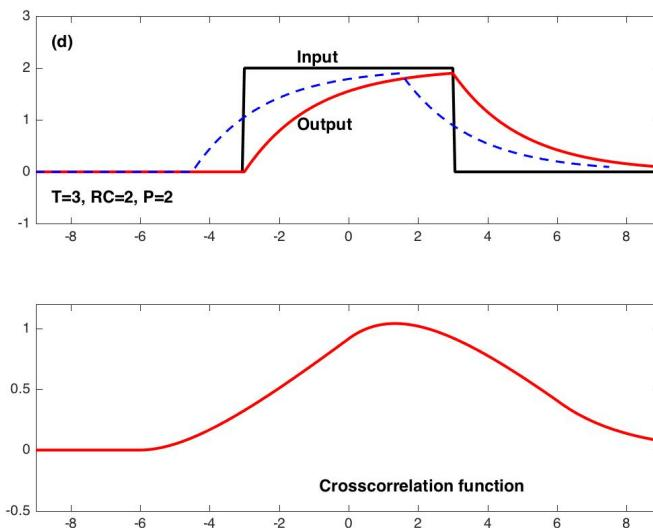
The input (b) and output (r) functions (top) with their associated crosscorrelation (bottom).
