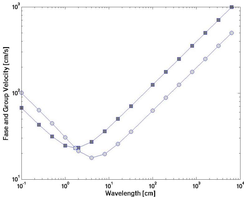
*Square symbols: phase velocity; circular symbols: group velocity; both are shown as function of wave length (on log-log scale). The phase velocity is minimal at  $\lambda = 1.7$  cm, the group velocity at  $\lambda \approx 4$  cm.*
