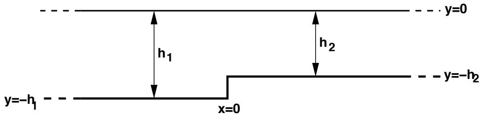
(a) We deal with reflection and transmission in  $x = 0$  when the impedances for  $x < 0$  and  $x > 0$  differ. For the impedance the following holds:  $Z = \rho \cdot v_\varphi$ . The density of the water is the same throughout, so we only have to look at the velocities in the two compartments. These are found from the dispersion relation:
