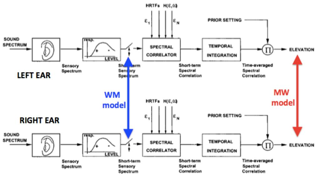
In the two different models of Fig. 8.19, here in extended format of Fig. 8.16, azimuth information enters the system either at the spectral input stage, where the spectral information from both ears is combined (WM model), or at the spatial stage where the elevation estimates of both ears interact (MW model).
